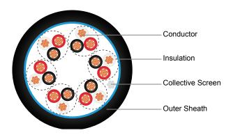
Conductor: Solid, stranded or flexible plain or metal coated copper in accordance with class 1, 2 or 5 of
