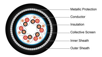
Conductor: Solid, stranded or flexible plain or metal coated copper in accordance with class 1, 2 or 5 of
