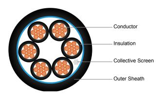
Conductor: Solid, stranded or flexible plain or metal coated copper in accordance with class 1, 2 or 5 of
